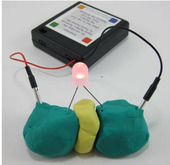
Figure 5. Your first play dough circuit should look like this.
